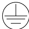
3872 – Earthing marking. The earthing marking in the drawing (connection side of the unit) shows the earthing point for earthing connection by customer. The earthing connections on the unit itself are also marked with this label (not shown in the drawing).
